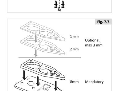
3. Put the five screws through the lock plate, the mandatory 8 mm spacer and the selected optional spacers (gray in picture) (Fig. 7.8).
